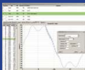
Waveform Analysis Shows harmonic content of metered waveform.
